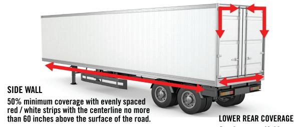
Continuous red/white covering 100% of the trailer width (doors) or horizontal bar surface (bumper).
