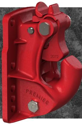
Certain coupling equipment parts, like pintle hitches and drawbar eyes, are already heat treated to withstand harsh environments and conditions.
