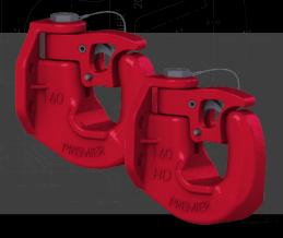
Max Gross Trailer Weight: 30,000 lbs. (13,607 kg) Maximum Tongue Weight: 4,500 lbs. (2,041 kg) Ultimate Latch Capacity: 5,000 lbs. (2,267 kg) Maximum Eve X-Section: 1 13/16 in. (46 mm) Minimum Eye Opening: 2 in. (51 mm) Unit Weight: 14 lbs. (6.4 kg)
