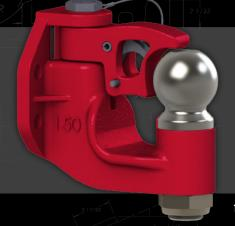
MGTW with Drawbar Eye: 20,000 lbs. (9,072 kg) MGTW with 155 or 156 Ball: 10,000 lbs. (4,535 kg) Maximum Tongue Weight: 2,500 lbs. (1,134 kg) Ultimate Latch Capacity: 5,000 lbs. (2,267 kg) Maximum Eye X-Section: 1 13/16 in. (46 mm) Minimum Eye Opening: 2 3/8 in. (60 mm) Unit Weight: 15 lbs. (6.8 kg)
